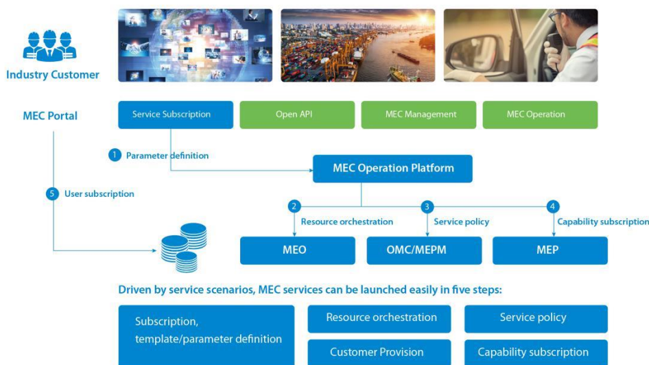
Figure 5-3 Automatic Onboarding of MEC Applications
